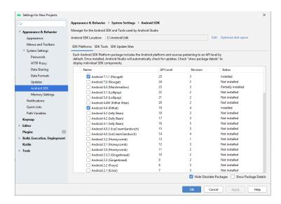
Debugging of Android applications is typically performed over the Android ADB USB interface. To enable this feature within Android Studio the USB debug feature must be installed in the Android SDK manager.
